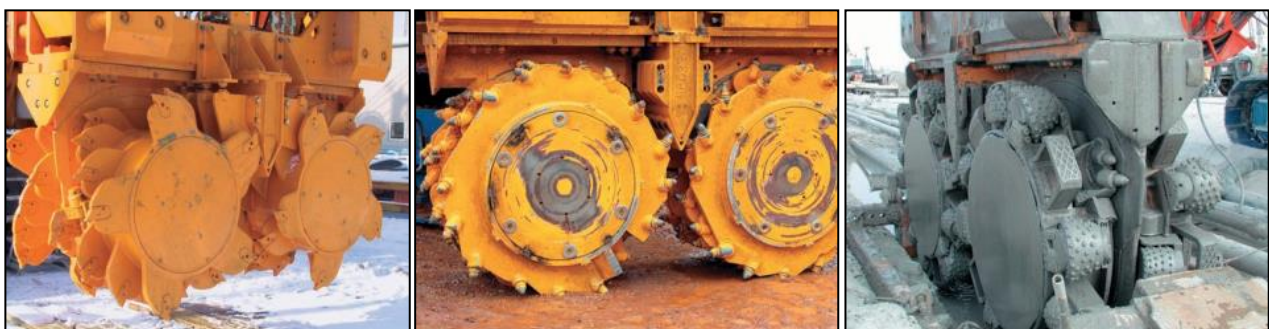
Figure 2. Standard Cutter Wheel (left), Round shank chisel cutter wheel (centre), Roller bit cutter wheel (right)
